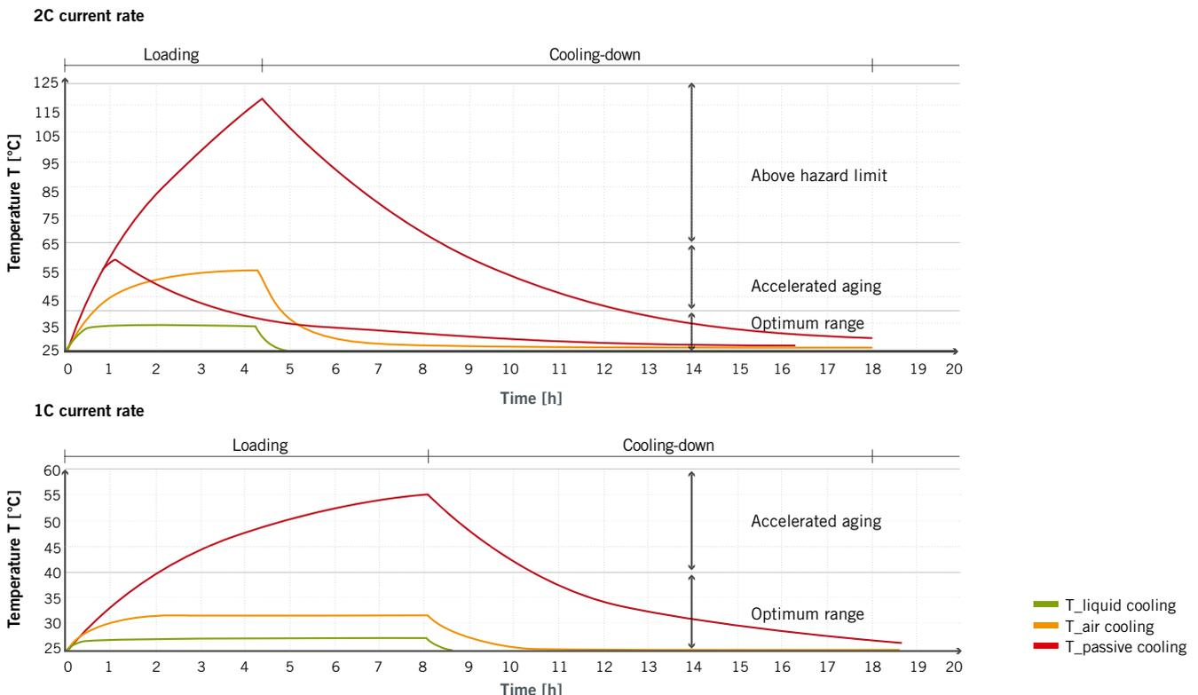
**FIGURE 4** Typical temperature variations for lithium-ion battery systems with different loads (1C and 2C current rates) and three kinds of cooling designs (© Akasol)
