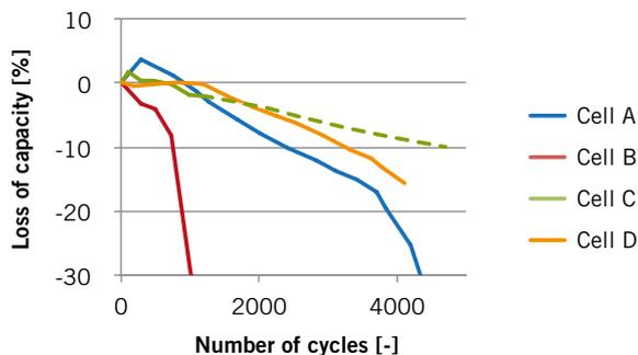
**FIGURE 1** Capacity of various lithium-ion cells in the course of a cyclical aging test (© Akasol)
