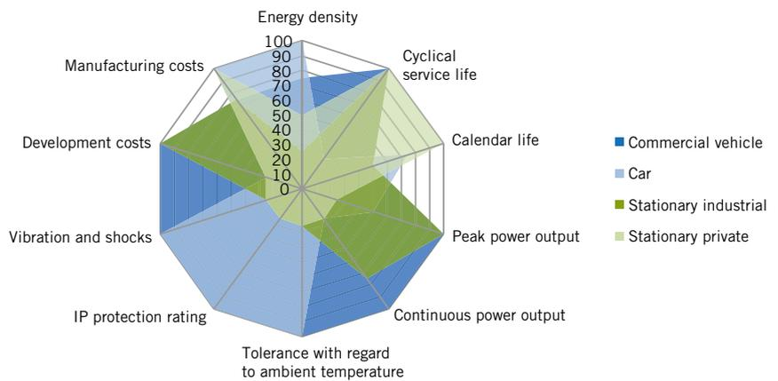
**FIGURE 3** Weighting of requirements in different applications (© Akasol)
