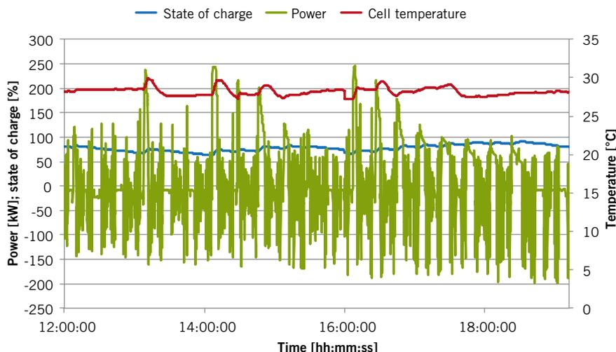
**FIGURE 5** Graphs of state of charge, power, and cell temperature over a loading profile derived from an application in a city bus (© Akasol)
