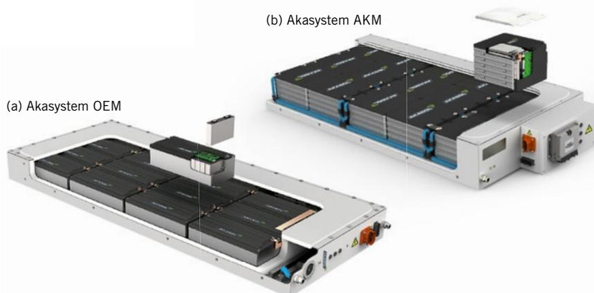
**FIGURE 6** Mobile battery systems for commercial vehicles: (a) OEM system with tested safety according to EUCAR, GB/T, UN 38.3 and ECE R100; (b) AKM system with tested safety according to USABC, IEC, SAE and UN 38.3 (© Akasol)
